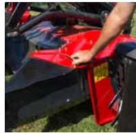
Integrated swath plates, easily adjusted to correct swath width.
