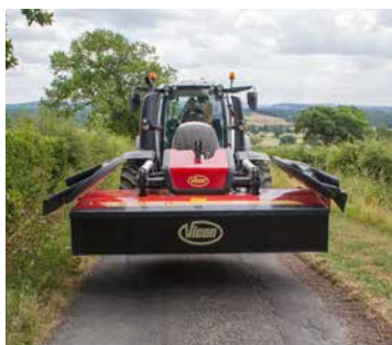
Hydraulic folding of FlexProtect guards (optional).
