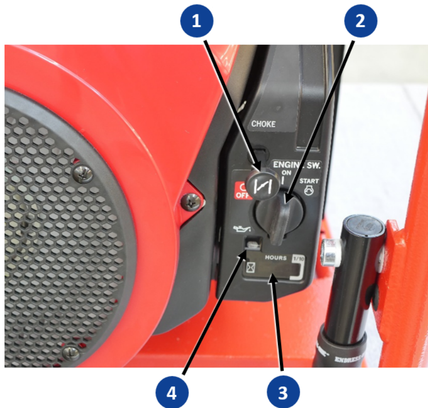
Fig. 7-2 Engine start on control panel
