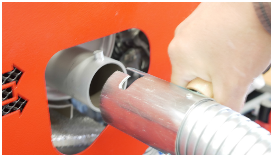
Fig. 8-5 Connecting up the exhaust hose
