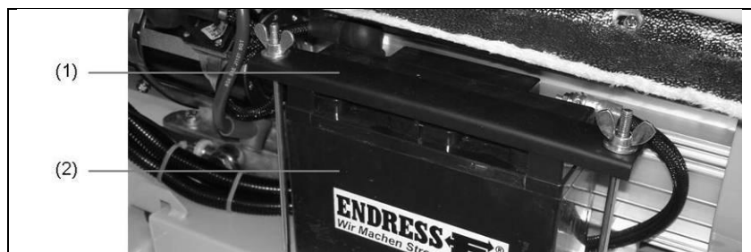
Figure 6-3: Replacing the battery
