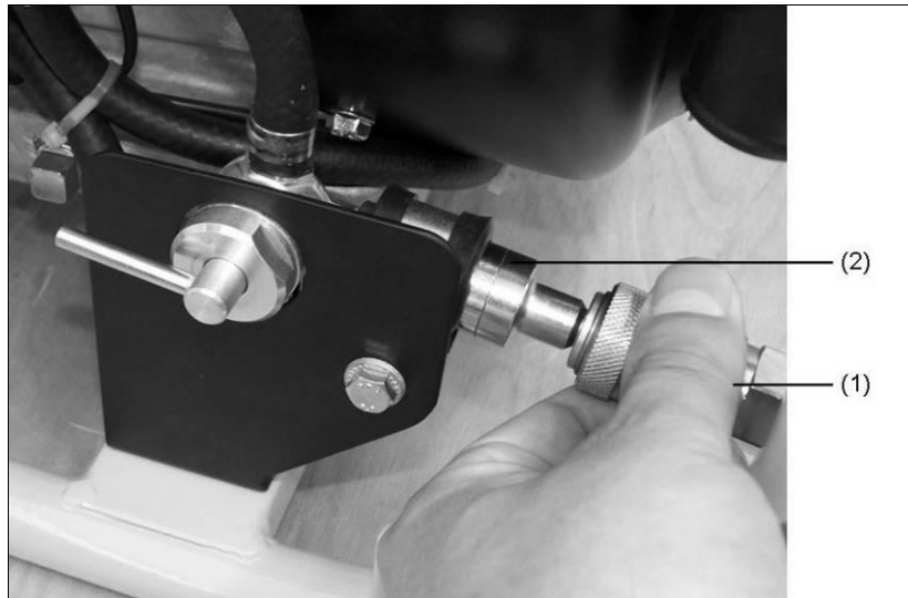
Figure 5-11: Connect up fuelling device
