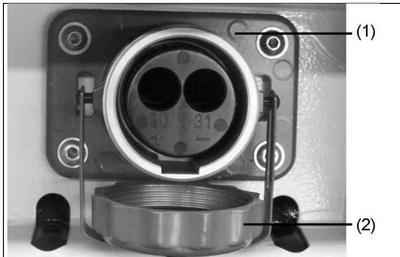
Figure 5-6: Connecting up an external start device
