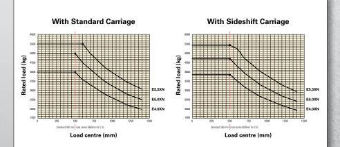
**Load centre:** Distance from front forks to centre of gravity of load. **Rated load:** Based on vertical masts up to 4 600 mm to top of forks.
