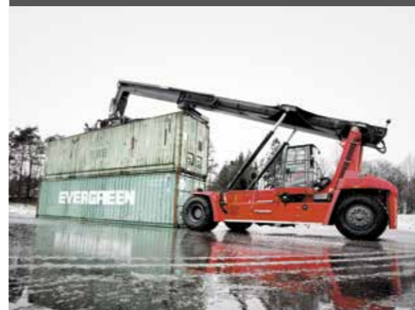
Precise lifting of long container end-on - 40 ft
