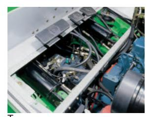
he hydraulic power steering unit is installed underneath the platform, giving simpler connections and quieter operation. The pedals are mounted on the dashboard for easy maintenance.
