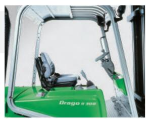
Ergonomically designed controls. The rotating-switch controlled parking brake is within easy reach of the driver. The new steering column is inclined towards the operator and easily adjustable for increased driving comfort.
