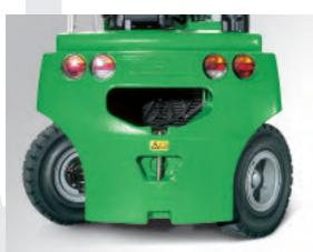
The wheels – which are among the largest in this class of trucks – guarantee load stability, operator's comfort and easy manoeuvring on uneven ground. Manoeuvrability is enhanced by a compact steering axle fully protected against the type of accidental impact damage typically associated with outdoor usage.
