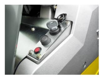
Simply use an ignition key to start the model with electric starter. A loud signal tone prevents inadvertent draining of the battery.
