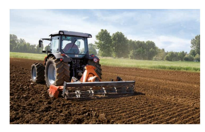
to 3,600 kg by adding additional lift rams. The button for proportionally controlling raising and lowering of the linkage arms facilitates implement coupling. For those requiring front-mounted implements, these tractors may also be equipped with a front linkage (with a load capacity of 1,750 Kg) and a 1,000 rpm front PTO: an attachment which will further extend the capabilities of the Dorado. It can also be used for carrying front ballast for the tractor.
