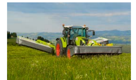
Compact hitch at the front linkage gives the mower generous ground clearance at headlands.
