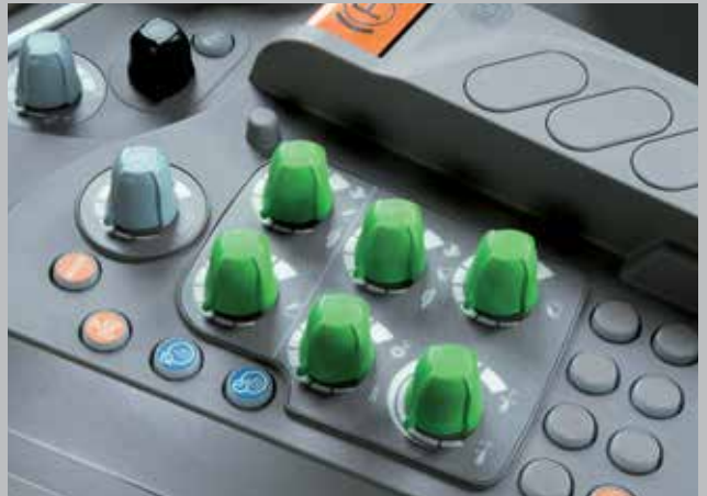
Fine tuning front (TTV only) and rear lift control can be operated through dedicated controls.
