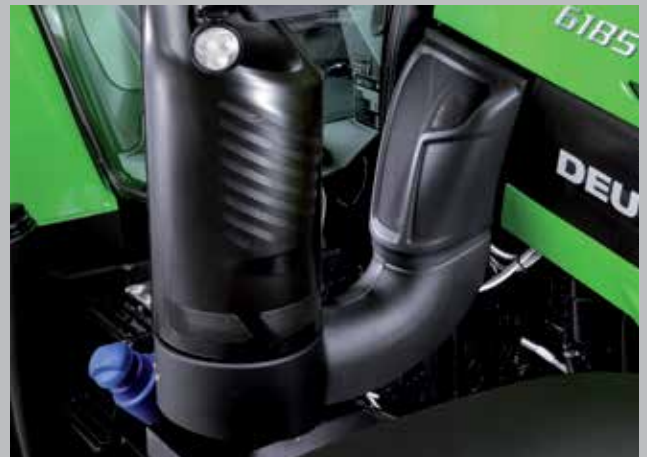
SCR after treatment system and passive DPF (diesel particulate filter) save fuel and costs.
