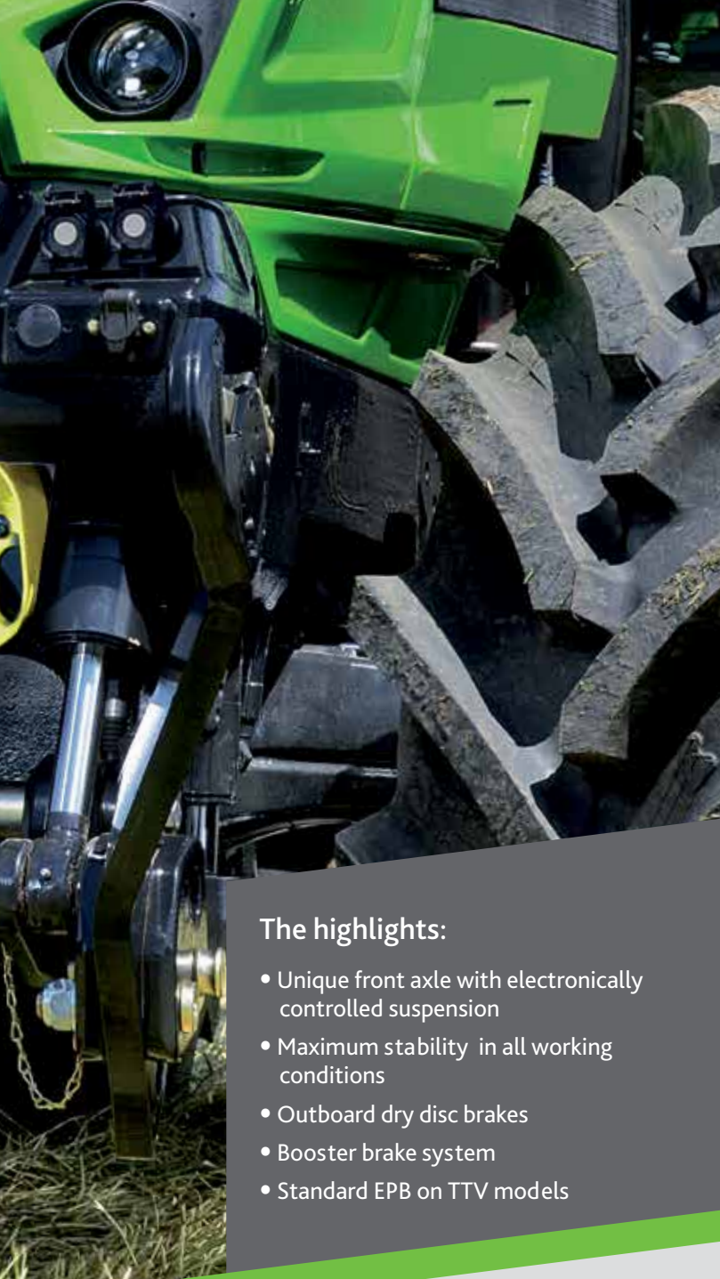
Electronic adaptive suspension incorporating an Anti-Dive and Anti-Rise system. The suspension can be used in the field and on the road. Fully lockable when needed.
