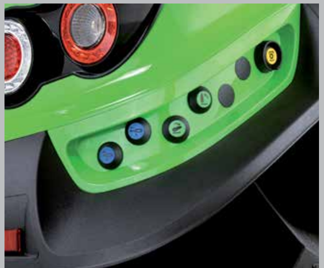
External hydraulic, rear lift and PTO remote controls from each side.
