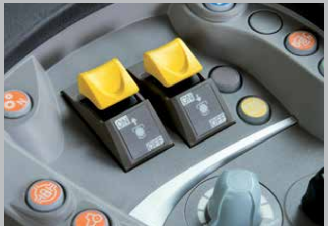
Standard in all cab configurations, the PTO engagement comes with the easy but safe push-button controls.
