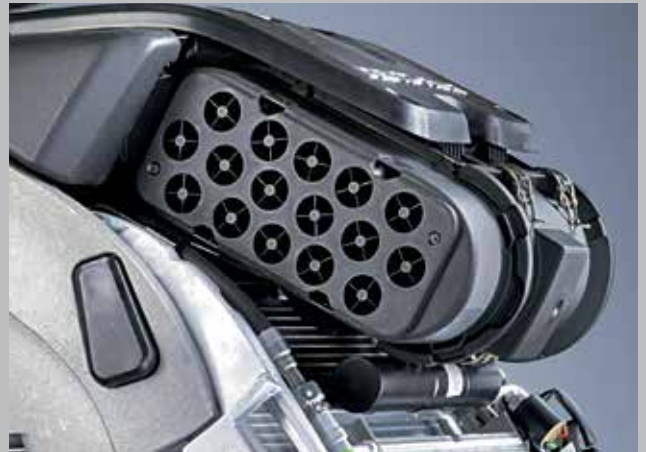
Precleaning system of the air intake filter: spiral tubes and an aspirator hose removes 95% of the dust before entering the primary filter.
