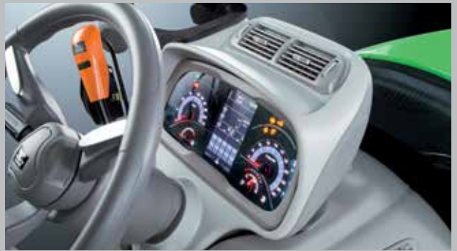
State-of-the-art dashboard cluster with new InfoCenter: 5" high-res LCD color display for customisable top information concept.
