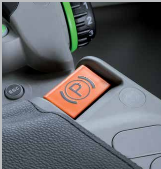
TTV models - EPB replaces the handbrake lever and is operated via an electric push-button control on the armrest console.
