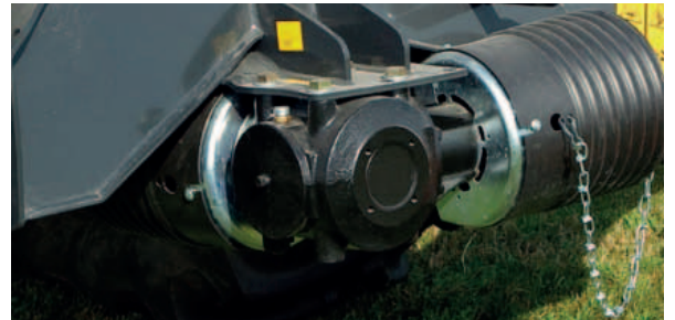
540/1000 rpm adjustable gearbox as standard.
