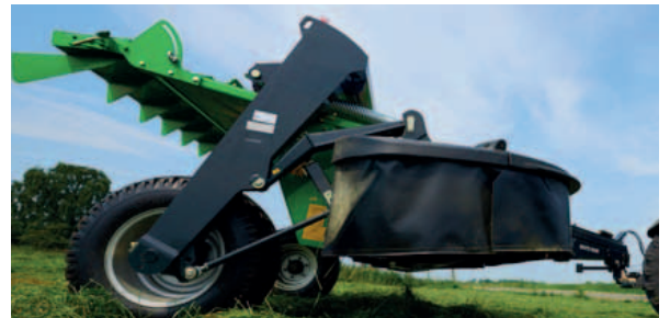
A lifting height of 50cm ensures excellent ground clearance for transport and during headland turning.
