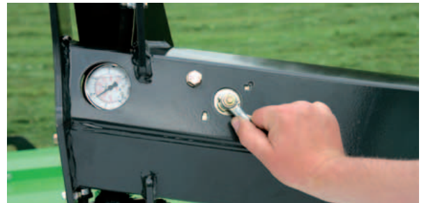
Hydraulic suspension for easy and precise setting of ground pressure.
