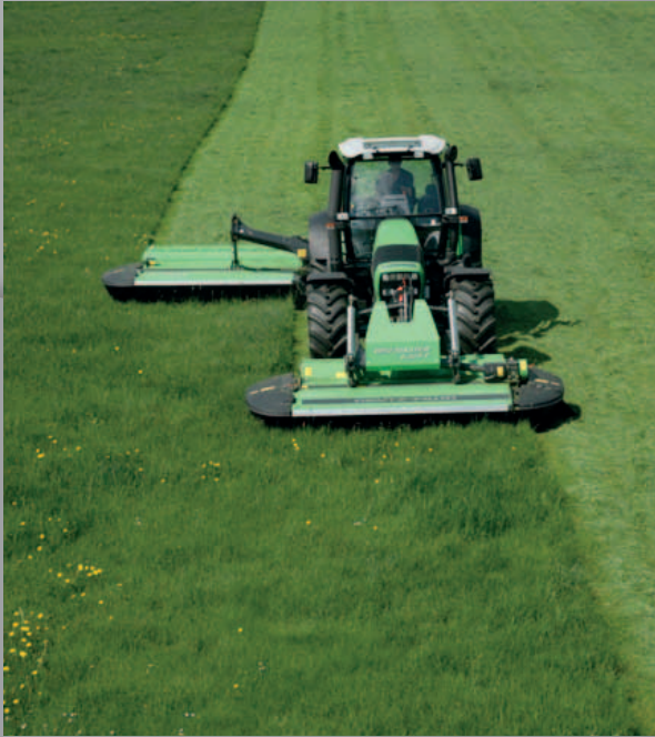
Mower combination with a working width of 6.2m.
