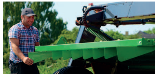
Dismount the two deflector doors and you are ready to mow.
