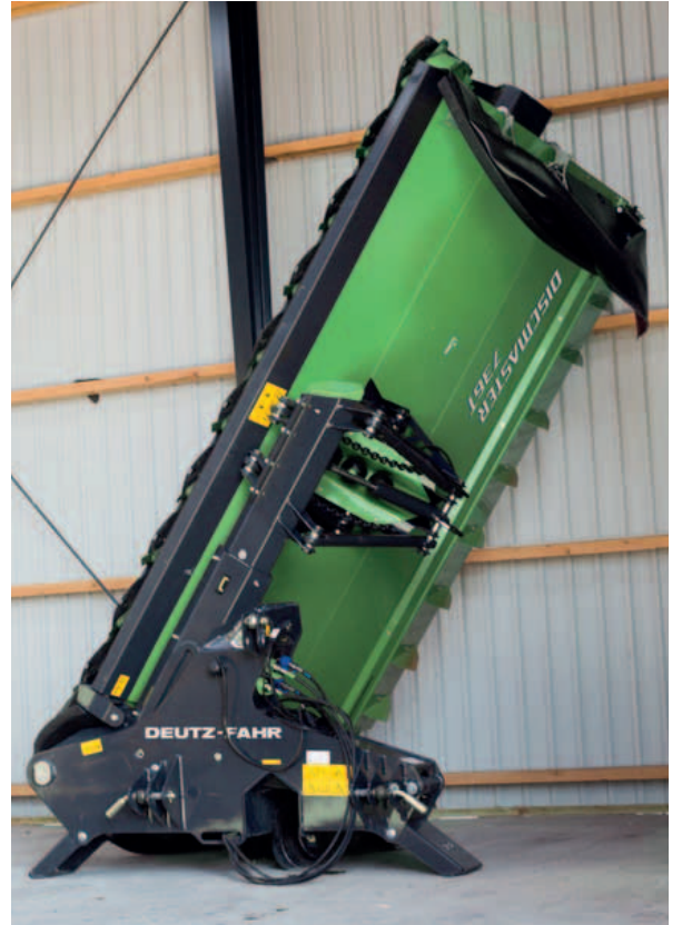
When parked, being in working position or during vertical storage the lift arms are always in a horizontal position, making it very easy to mount or unmount the mower from the tractor.
