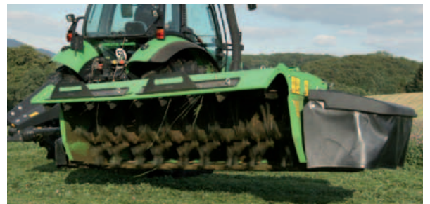
Easy lift on headlands without activating the 3-point linkage of the tractor.
