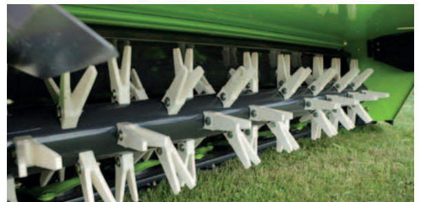
Effective 600/900 rpm nylon tine conditioning.
