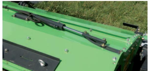
The left hand side swath plate can be adjusted hydraulically from the tractor cabin (option).
