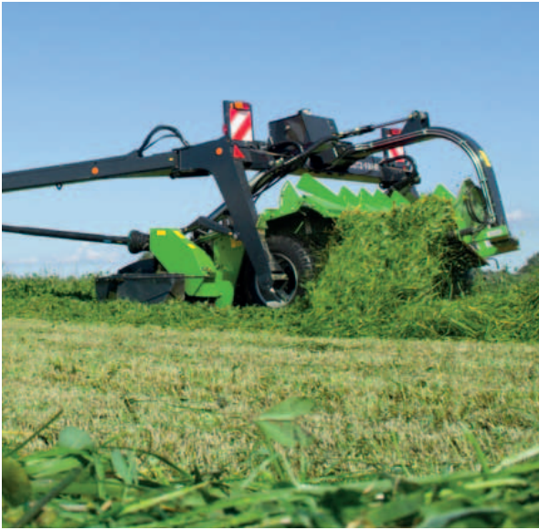
The DiscMaster 900, fitted with the versatile swath belt, allows you to place two swaths together.
