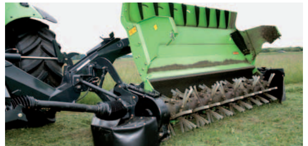
The complete end of the mower can be lifted to give easy access to the conditioner.
