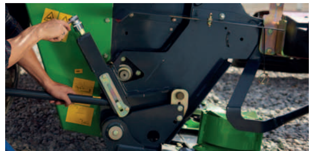
Easy adjustment of stubble height.
