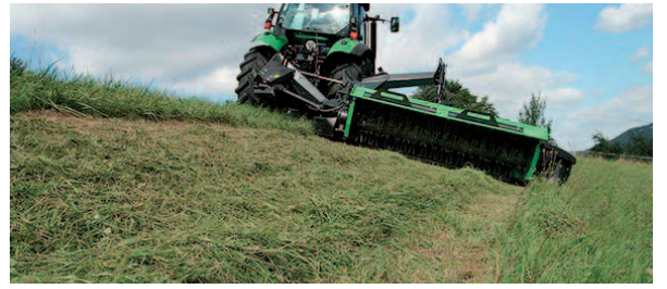
The mown crop is moved away from the ditch, making it very easy to collect afterwards.
