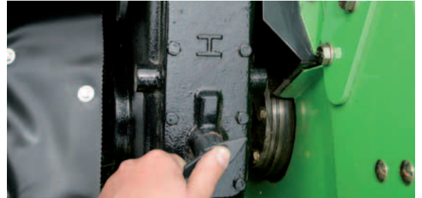
Conditioner speed of 900 or 600 rpm - changed in a second.
