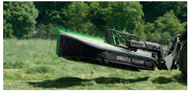
Minimum 500mm ground clearance across the complete mowing unit during headland turns.
