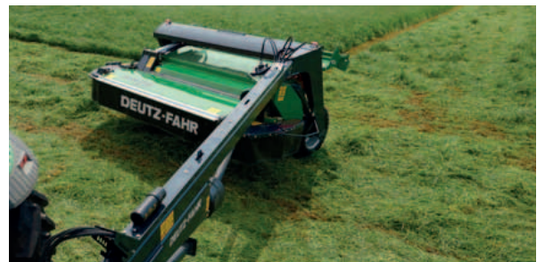
The swivel hitch headstock, with reversible gearbox, provides optimal manoeuvring ability.
