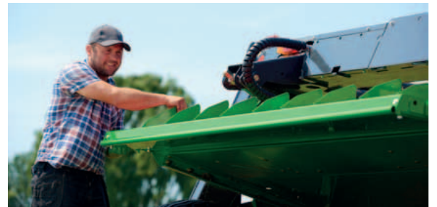
Setting DiscMaster 900 series mowers for wide spreading is very simple. Simply turn the rear plate 180°.
