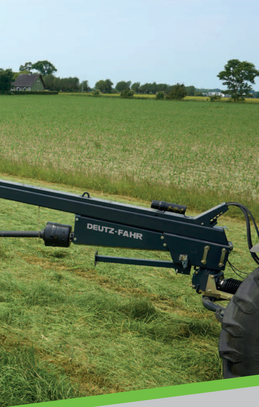
The swivel hitch headstock, with reversible gearbox, provides optimal manoeuvring ability.
