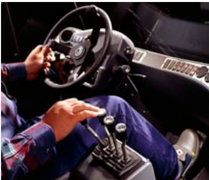
Hydraulic or electric servo control by levers.
