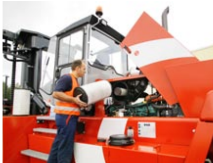
The air filter is easy accessible under the bonnett.
