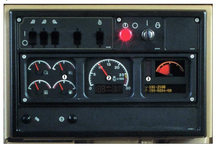
**The Vital Information Display System (VIDS)** provides the operator with continuous feedback on machine and system operation, and includes three levels of operator alert.
