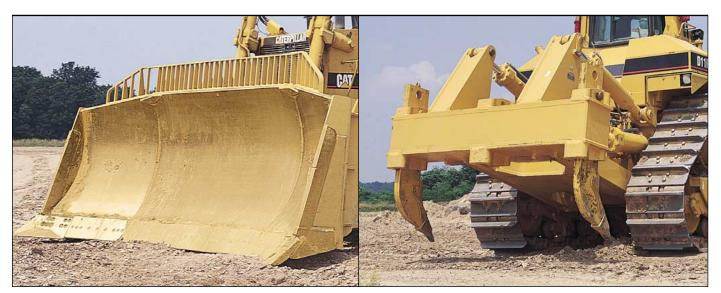
**Bulldozers.** The 11SU blade, rated at  $27.2 \text{ m}^3$  ( $35.5 \text{ yd}^3$ ) and the 11U blade at  $34.4 \text{ m}^3$  ( $45.0 \text{ yd}^3$ ) make full use of D11R power.
