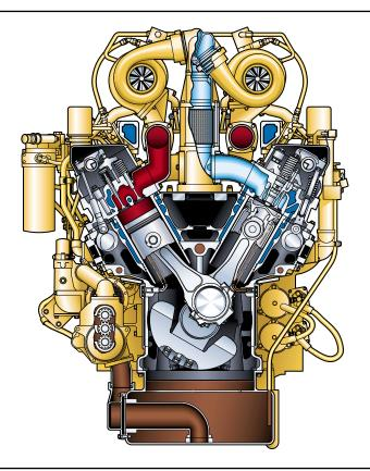
Caterpillar® 3508B Diesel Engine with Electronic Unit Injection (EUI) performs at rated net power of 634 kW (850 hp) at 1,800 rpm with a torque rise of 25 percent and meets worldwide emissions regulations for the Environmental Protection Agency (EPA), the European Union (EU) and the Japan Ministry of Construction (JMOC).
