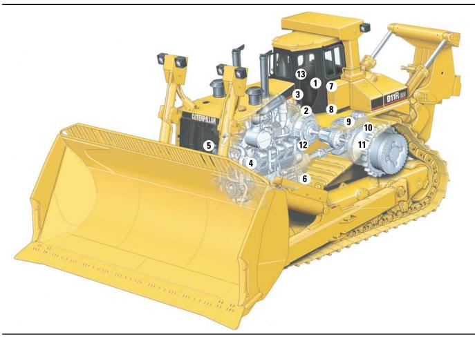
**By communicating,** these components work to optimize overall power train performance, reliability and component life for reduced power train operating cost.
