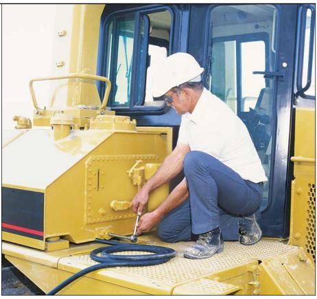
**Ecology drains** provide an environmentally safer method to drain fluids. They are included on the radiator, hydraulic tank and major power train components.
