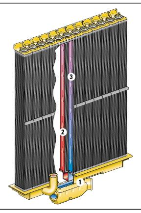
Advanced Modular Cooling System (AMOCS) utilizes an exclusive two-pass cooling system and increased cooling surface area to provide significantly more cooling capacity than conventional systems.
