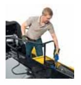
The fuel and 120 litre AdBlue tanks are conveniently located next to each other to facilitate simultaneous filling.
