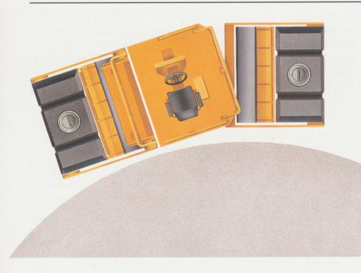
**Off-center articulation** with 60% of the machine length behind the pivot and 40% forward.
