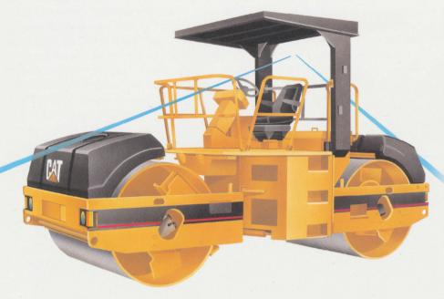
**Visibility to objects** 1 m (3.3') high and 1 m (3.3') in front of the machine or behind the machine.
