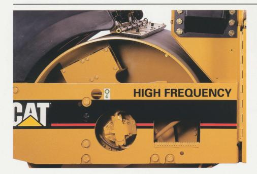
**High frequency allows faster travel speed** at the specified impact spacing.
