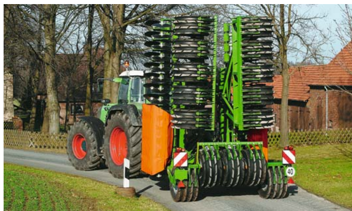
Trailed, hydraulic folding Catros with wedge ring tyre roller in 7.5 m working width.
