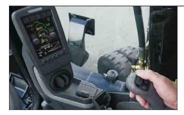
**Tool Control.** Ten hydraulic pump flow and pressure settings can be preset within the monitor, eliminating the need to adjust the hydraulics each time a tool is changed. Selecting the proper setting from the monitor menu instantly provides the operator with the correct amount of flow and pressure for the tool.
