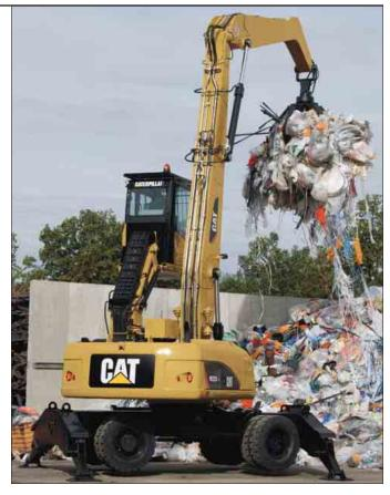
**M318D MH Sticks.** Two options of MH sticks are available for the M318D MH, all equipped with high and medium pressure auxiliary lines. The 4900 mm Drop Nose Stick offers the reaching and lifting capabilities required for typical MH applications, while the 4200 mm Straight Stick is the best solution for when additional work tool functionality is needed.
