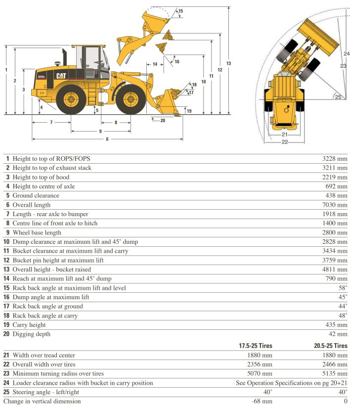
Dimensions listed are for 924Gz with optional counterweight, standard lubricants, full fuel tank, cab with A/C, sliding glass, Cat contour seat, limited slip axles with dual disc rear, 4L 4V hydraulics, heavy duty cooler, supplemental steering, roading fenders, reversing fan, back-up alarm, guards, ride control, radio, 1.8 m³ bucket with bolt-on cutting edge, 80 kg operator and 20.5 R25 radial (L-3) XHA tires. Refer to Operating Specifications for bucket variations.
