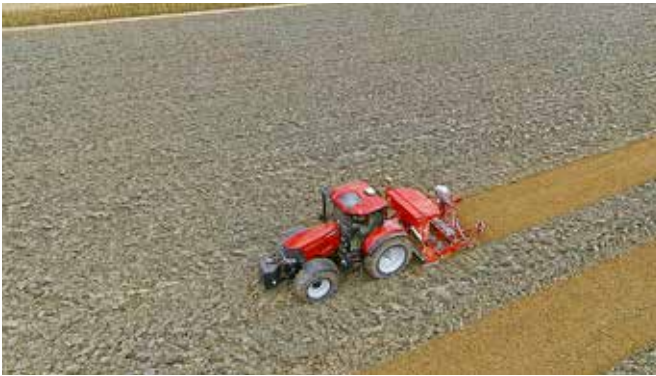
AFS AccuGuide: GPS and GLONASS based guidance for ultimate precision independent of crop conditions. With RTK accuracy levels down to 2.5 cm available.
