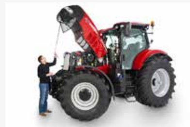
EASY ACCESS The single-piece engine hood is raised using a gas strut and can be locked at an angle of 45° and 90°, even with front attachments fitted.
