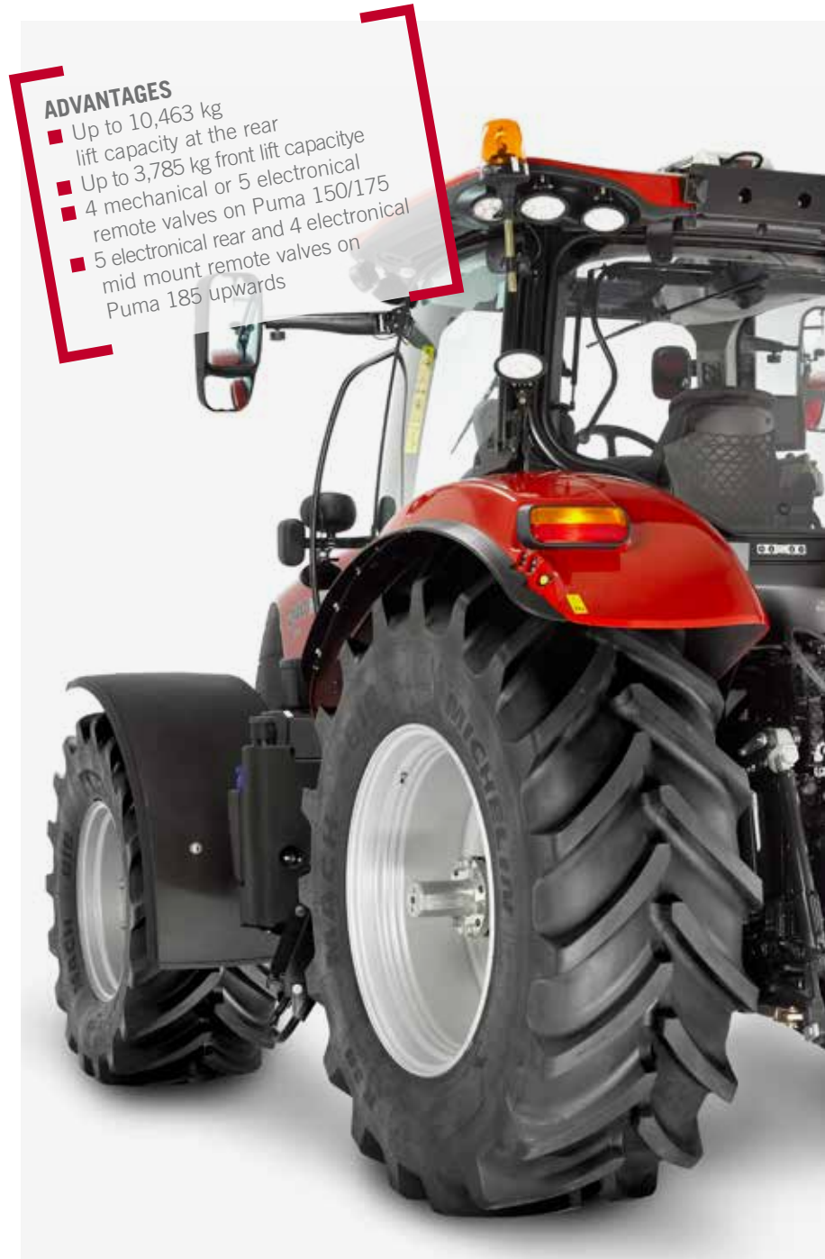
No limits of operation with 5 electronic-hydraulic rear remotes.
