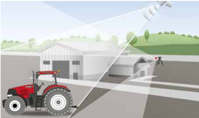
xFill bridges RTK signal gaps of up to 20 minutes.
