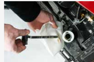
FAST DAILY CHECKS The engine oil can be checked and topped up when the bonnet is closed.
