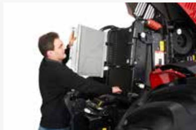
CLEANING COMPLETE IN NEXT TO NO TIME The radiators can be swung out to enable easy cleaning.
