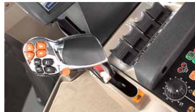
Multicontroller™ allows gear change without actuating the clutch.
