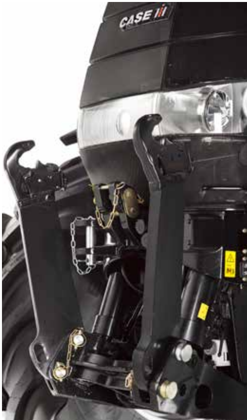
Seamlessly integrated Front Linkage with a lifting power of up to 3,785 kg.
