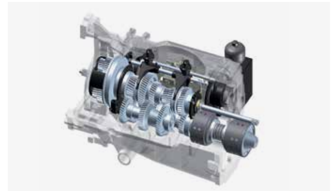
CVX transmission – stepless drive between 0-50 kph
