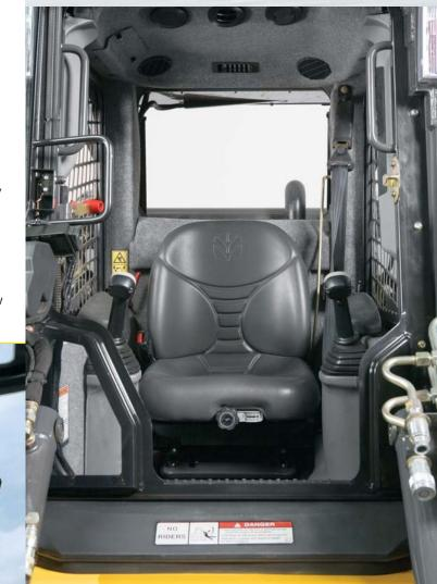
Adjustable contoured armrests and suspension seat allow operators to find a comfortable working position.
