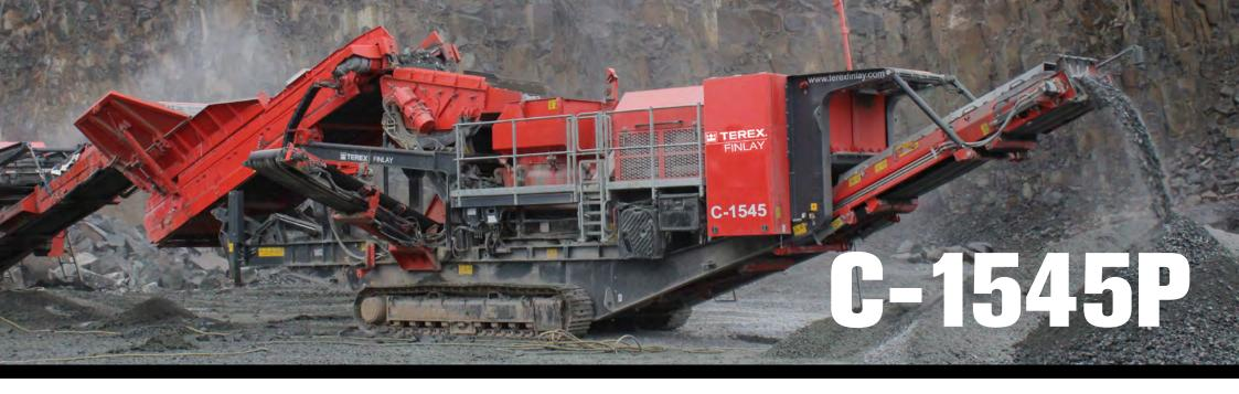
The Terex® Finlay C-1545P incorporates the Terex 1150 cone crusher driven through by direct clutch drive with variable speed, automatic tramp relief and hydraulic closed side setting (CSS) adjustment.
