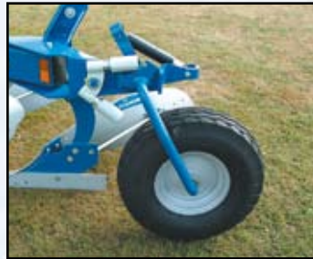
Pendelend, rubberen steunwiel (7.00 -12). Diameter 645 mm en 182 mm breed.
