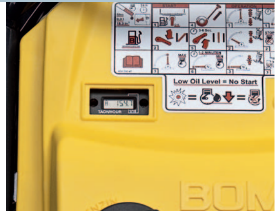
Hour counter and tachometer with service display for regular service planning.
