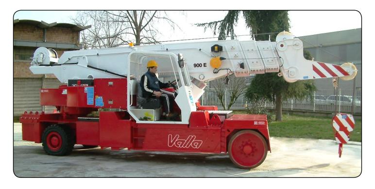
**PROPULSION:** 48 kW - 96 V DC fanned reversible electric motor fitted with a MOSFET speed control and microprocessor.
