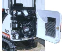
The tailgate latch is hidden, and opens with a lever located in the operator area. (The upper structure of the excavator is also made of quarter-inch steel for superior strength in all applications.)
