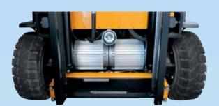
Twin-motor traction and lift motor with MONTINIplus electronic technology in Alternating Current (AC).
