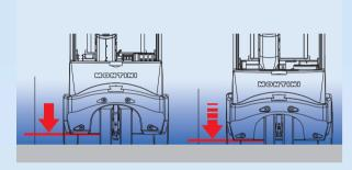
When the speed exceeds 12 km/h, a microprocessor operates the suspension lowering.
