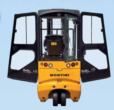
The model BINGOplus N 163 GA can be equipped with battery up to 48V/640Ah. The model BINGOplus N 183 can be equipped with battery up to 48V/750Ah.
