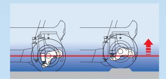
When the truck is running on uneven surface, the suspension reduces by 20% the vibrations transmitted to the driver's body. Effort and occupational diseases are reduced this way. In addition, the suspension reduces those tensions, vibrations and shocks that cause damage to the mechanical and electrical components.
