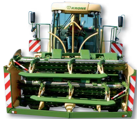
Compact transport position: The triple-fold EasyCollect header
