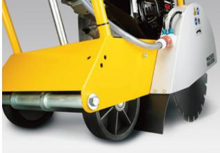
The gasoline-driven floor saw models BFS 1345 and BFS 1350 are available with either a standard or shortened wheelbase. Even better maneuverability of the floor saw can be achieved with the shorter wheelbase.
