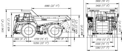
\*Overall dimensions are specified for standard equipping of the dump truck
