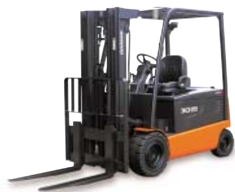
B22X / B25X / B30X / B35X-5 2,200kg to 3,500kg Capacity Pneumatic Tire
