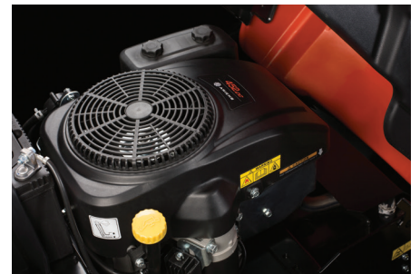
The E36 features a highly reliable, single cylinder 452cc Ariens engine
