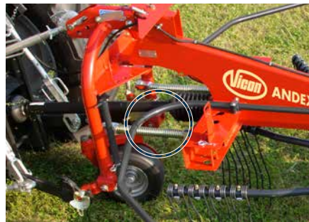
Oscillation dampers ensure excellent running characteristics.
