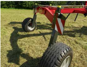
Active wheel steering for improved manoeuvrability in combination with large wheels for reduced compaction.
