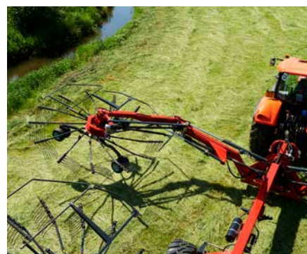
The two outer rotors can be adjusted individually to match a working width between 9.8-15.0m.
