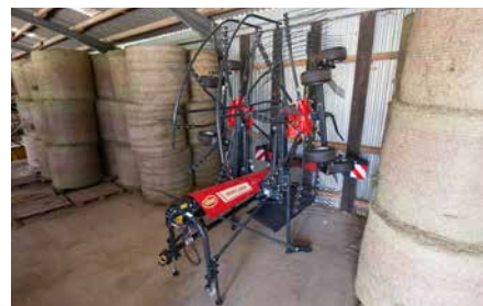
More flexibility by parking as no tine arms need to be detached.
