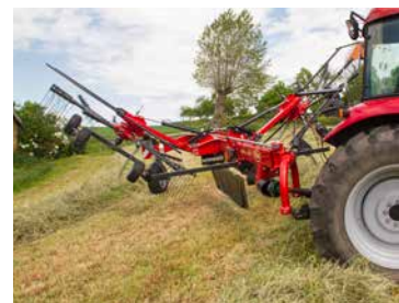
Active wheel steering and sharp turns up to 80°.
