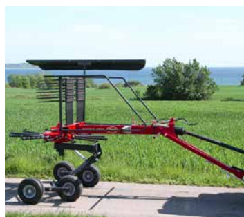
With a linkage mounted drawbar, the Andex 474T can be easily operated by low horse power tractors.
