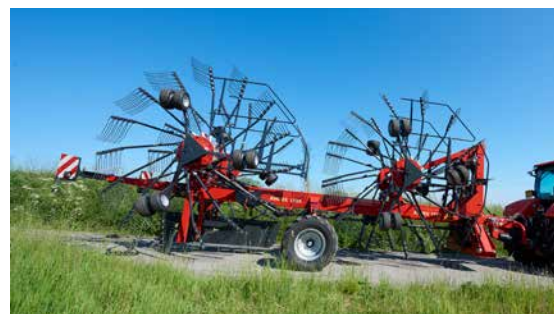
Vicon Analex 1505 Clever folding mechanism for road transport.
