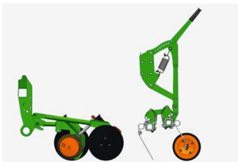
Roller bar in operation: the drag tine harrow covers the seed with soil which is then pressed by the Roller harrow.
