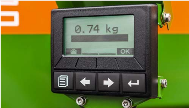
Calibration via the TwinTerminal 3.0
