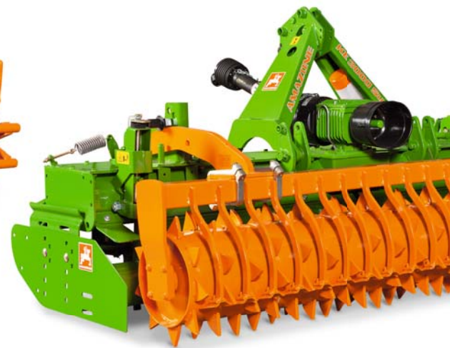
KE 3000 Super with 500 mm tooth packer roller
