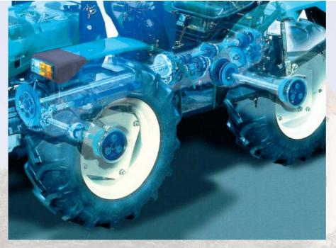
mechanical or electro-hydraulic control, can be inserted as needed to maximize traction.
