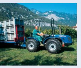
VALIANT tractors are available in conventional mono-directional versions and in reversible versions where the driving position (seat, steering wheel, dashboard) can be reversed in just 5 seconds without having to detach any connections.
