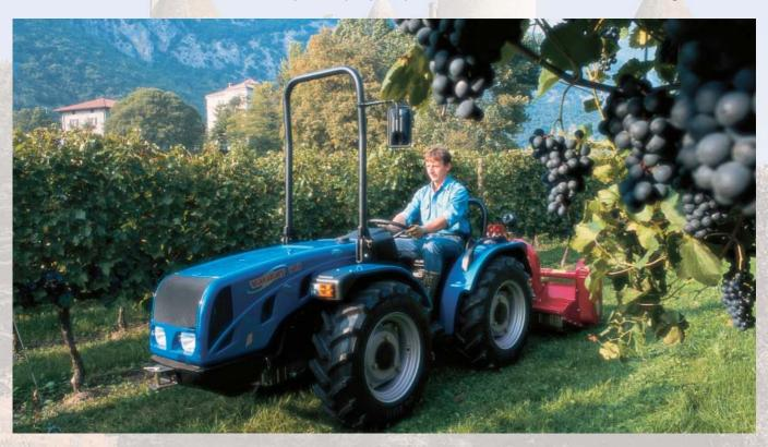
The optimal steering radius, the four wheel drive and the ideal weight distribution let you work safely and efficiently in difficult terrain. The comfortable driving position, the ergonomically positioned controls and the practical, easy to read instrumentation let you work without fatigue.
