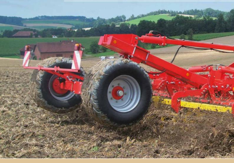
The length and inclination of the drawbar are adjustable. An ideal match to every tractor and rear roller is ensured as a result. This optimised mounting geometry improves ground clearance at headlands and during transport.
