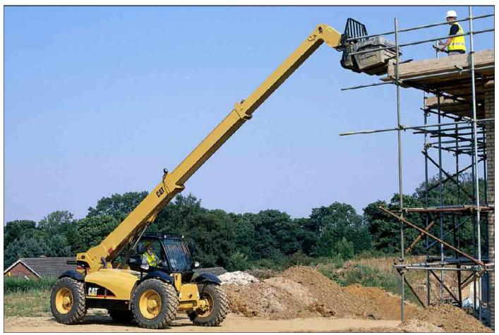
**Lift Height**. The TH340B can effectively and quickly place bricks, roofing materials and trusses to a maximum height of 9500 mm.
