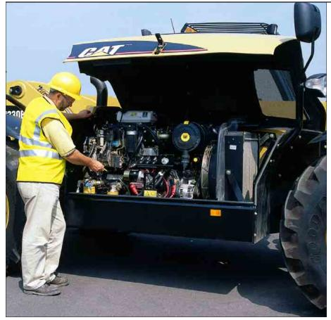
Access. All Cat Telehandler service points, including the combined transmission/hydraulic oil filter, are readily accessible and major components are easy to reach at ground level due to the overall machine design. A cab mounted service point allows access to the fuel fill, hydraulic oil fill, washer bottle, fuse box and cab air filter for daily checks. **Selection**. Make detailed comparisons before you buy. Your Cat Dealer can give you precise answers to these questions.
