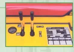
the operator can check the travelling speed by operating the throttles positioned on the side and he/she can sound the horn. The safety level is guaranteed by a device located on the control head unit that reverses the travelling direction in case of contact with
