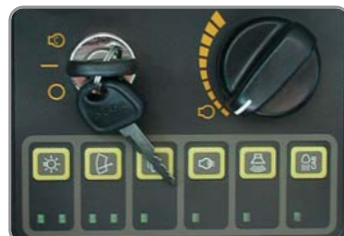
1 2 3 ① Wide, Comfortable Operating Space ② Steel Cover Sunroof ③ Dial Type Engine Speed Switch and Key Switch
