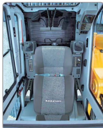
1 2 3 ① Wide, Comfortable Operating Space ② Steel Cover Sunroof ③ Dial Type Engine Speed Switch and Key Switch
