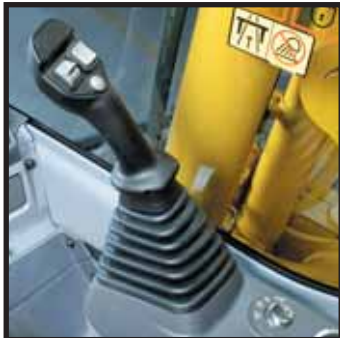
Joysticks with proportional control button for attachments
