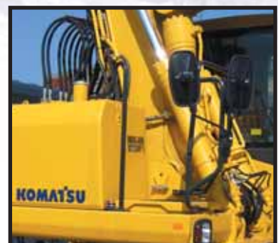
Large handrail for safe access
