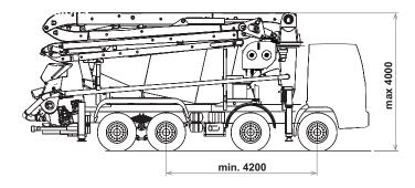
Dimensions varying according to truck assembly
