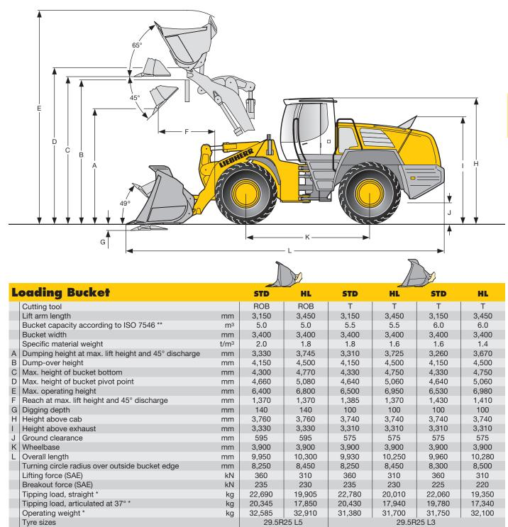
The figures shown here are valid with tyres above, includes all lubricants, a full fuel tank, the ROPS/FOPS cab and the operator. Different tyres and optional equipment will change the operating weight and tipping load.
