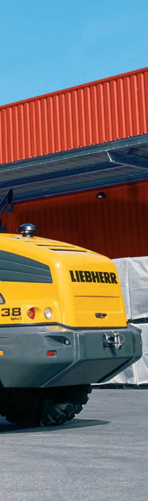
The Liebherr driveline enables the diesel engine to be installed in the ideal position. For this class of wheel loader, it is transversely mounted at the rear. This greatly increases the tipping load and the handling capacity per operating hour at a lower operating weight than conventional wheel loaders.
