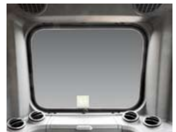
Rear Window Emergency Exit
