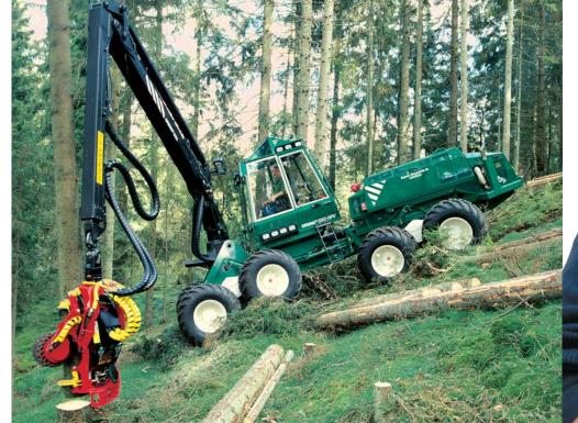
Unique longitudinal stability allows the HPV to operate at full capacity even on steep downhill slopes.
