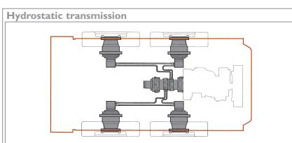
The gearboxes, compared with the traditional transmission by chain, which is subject to frequent repair and maintenance operations, have many advantages such as on elevated transfer speed, homogenous distribution of the power directly on the wheels in favour of the force, a higher sensibility in the movements, the favourable possibility to work if need be, mounting old and new tyres on the same side without compromising the reliability of the machine.
