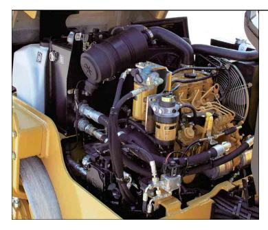
**Power.** The liquid cooled, three cylinder C1.5 engine provides a gross power of 24.6 kW (34 hp) for good performance and reliability in all working conditions.
