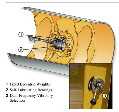
**Dual Frequency Vibratory System.** The standard vibratory system incorporates two frequencies of 63 Hz and 55 Hz in order to provide increased application versatility.
