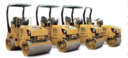
**CB22.** The CB22 is equipped with a 1.00 meter drum that provides a good balance of weight and power for good performance in tough applications.
