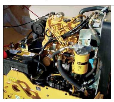
**Power.** The liquid cooled Caterpillar C1.1 engine provides a gross power of 16.1 kW (22 hp) at 2400 rpm for excellent performance with low sound levels maximizing operator comfort.
