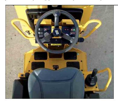
**Isolated Operator's Station.** The fully-isolated and roomy operator's station provides optimum operator comfort for day-long productivity. Rubber mounts on operator platform and seat reduces the vibrations transmitted to the operator, console and steering wheel.
