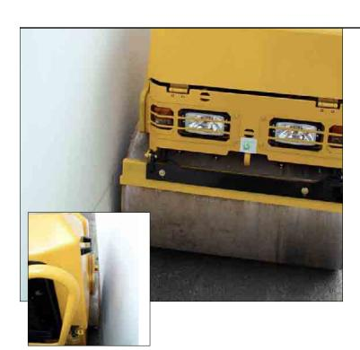
**Full flush compaction.** The front 900 mm offset driving drum allows the compactor to operate against a wall, curb or other vertical obstructions achieving complete compaction coverage.
