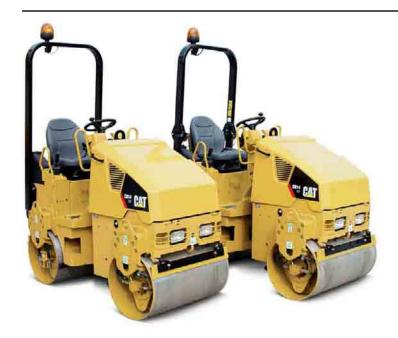
**Increased Production.** The CB14 XW is available in two versions; 900 mm wide drums and 1000 mm wide drums. These two versions enable increased mat width coverage in fewer overlapping passes.
