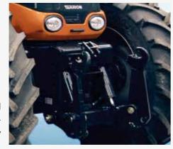
Powerful front system for attached implements and front power takeoff shaft, optionally
