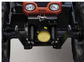
Powerful front system for attached implements and front power take-off shaft, optionally
