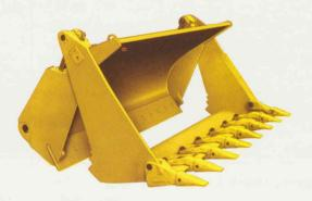
**Multi-Purpose bucket** gives versatility with strength. It loads, strips topsoil, bulldozes and cleans up debris. The bucket clamps hydraulically to grip logs, carry pipe or handle other tough-to-grasp materials. Options: teeth with Corner Guard System, bolt-on reversible cutting edge group, or bolt-on teeth and edge segments.
