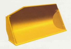
**General Purpose bucket** features high-strength, low-alloy steel plate for resistance to dents and abrasions. Shell tine assembly in bucket floor increases structural strength. Integral spill plates improve load retention.
