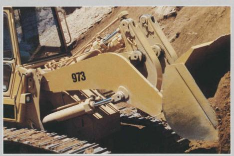
■ Faster dump speed . . . dump oil flow is into tilt cylinder rod end rather than head end — provides greater speed and faster response.
